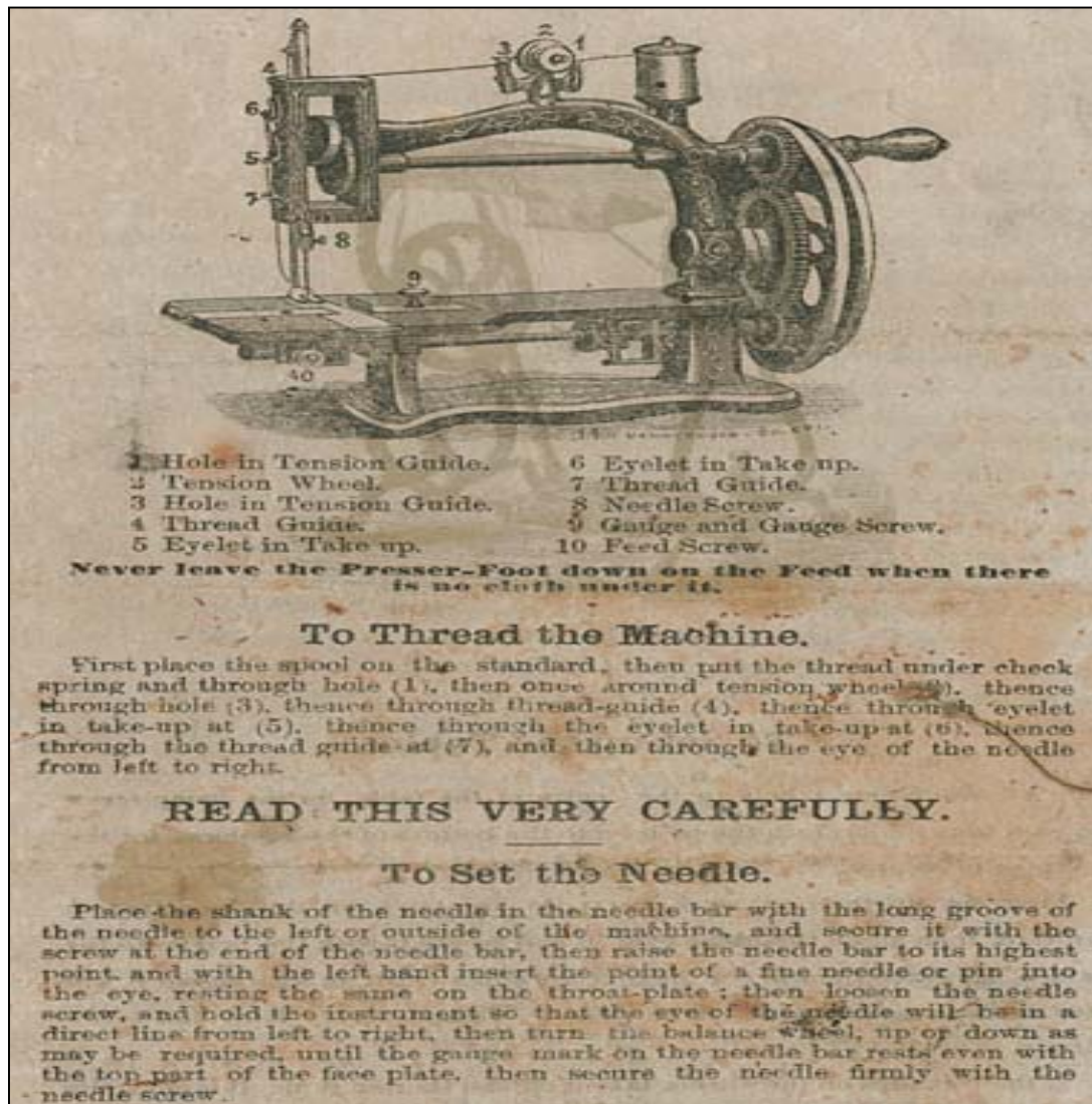
Fig. 3: Directions for Using the New Buckeye Under-Feed Sewing Machine (Wilson Sewing Machine Co. 1870: 4)
